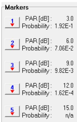
The **Markers** area at the bottom left part of the screen contains five result lines for the five markers on the CCDF display.
