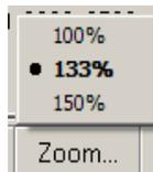
The **Zoom...** button allows for scaling the display of constellation points to 100%, 133% and 150%. 100% display concentrates the constellation in the middle of the screen but shows also pixels which appear far away from the centre points. The other modes give a more detailed display of the data carriers.
