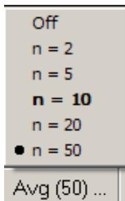
**Avg(.n.)** is active at MER vs Carrier and EVM vs Carrier measurements. The value in brackets on the button shows the actual setting.
