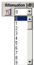
The **Attenuation [dB]** drop-down list enables you to set the input attenuator of the receiver in order to attenuate strong input signal levels or temporarily simulate lower field strengths.
