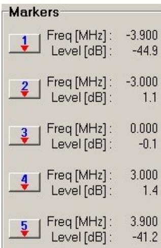
The **Markers** area at the bottom left part of the screen contains 5 result lines for the 5 markers on the spectrum display
