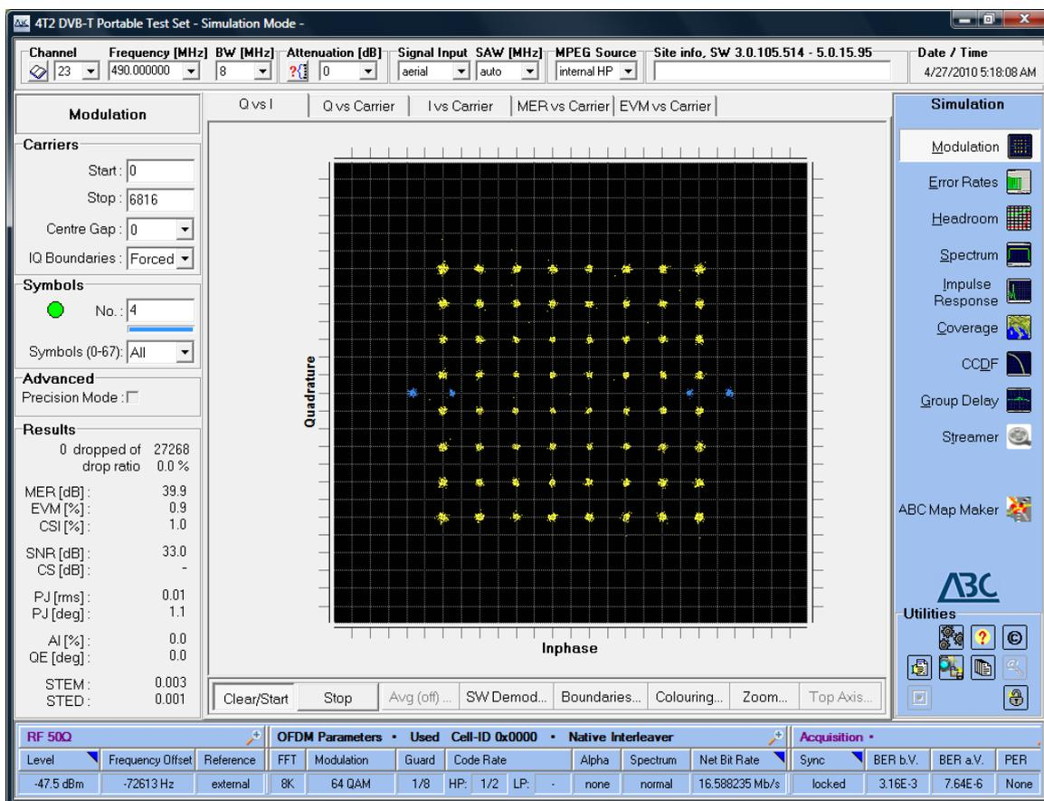
Illustration 11: /Analysis/Modulation/Q vs I display (constellation diagram)
