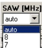
The **SAW** drop-down list selects the surface acoustic wave filter setting in the aerial input:
