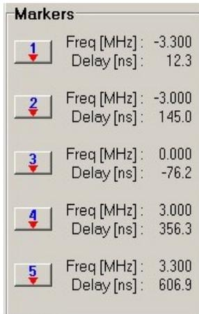
The **Markers** area at the bottom left part of the screen contains five result lines for the markers on the Group Delay display.
