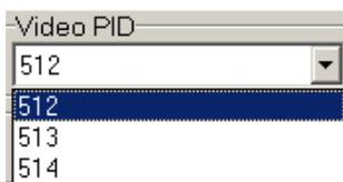
If you know the exact **PID** (Packet Identifier) of any program you wish to display, it may be more convenient to select this program by simply entering this PID directly in the **Video PID** or in the **Audio PID** combo box.
