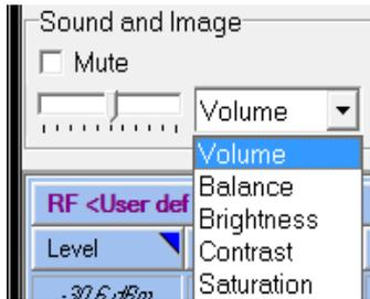
The **Sound and Image** section allows to fine tune the brightness, contrast, and colour saturation of the monitor.
