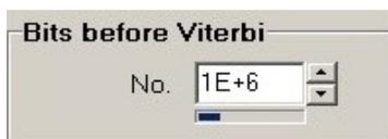
Fastest results; BER values down to  $1 \times 10^{-6}$  can be measured.
