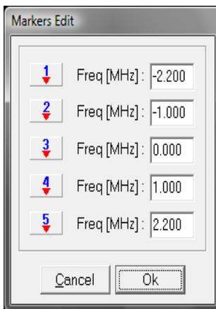
Instead of displaying the delay of a certain marker, you can click the arrow underneath e.g. the figure 1 marker to open the Markers selection dialog.
