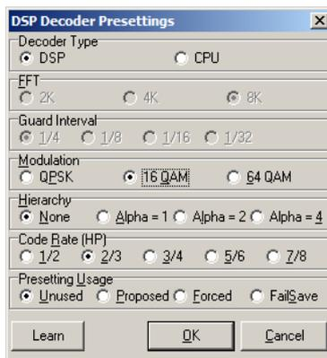
Is used to select between decoding by Chipset-DSP (hardware decoding) or by the internal computer CPU (software decoding).
