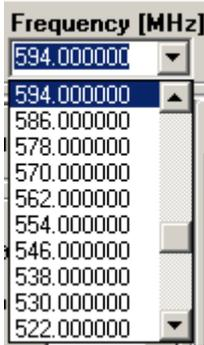
The **Frequency** drop-down list displays the centre frequency for the channel selection made from the **Channel** drop-down list.
