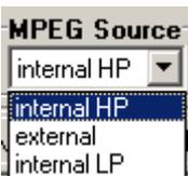
The **MPEG Source** drop-down list selects the source of the built-in MPEG hardware decoder, or Streamer Server:
