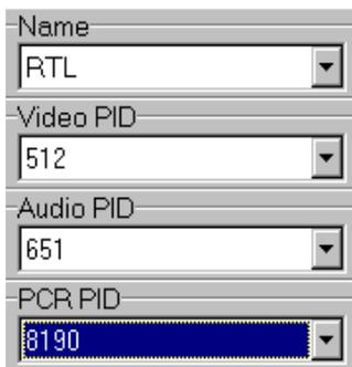
The four drop-down lists in the MPEG Video section enable you to make individual PID selections from the data available within the received DVB-T ensemble.
