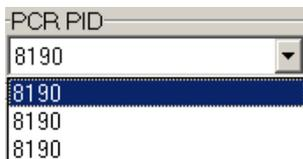
The **PCR** (Program Clock Reference) PID is required to synchronise audio information with the relevant video information of a TV program. Unless you change the PCR PID selected by default, the audio signal corresponding to a certain video signal will automatically be synchronised.
