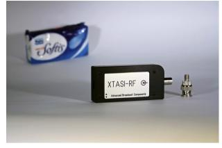
**XTASI-RF** is a pocket-sized **DVB-T/T2** receiver-input device in a robust aluminium housing.
