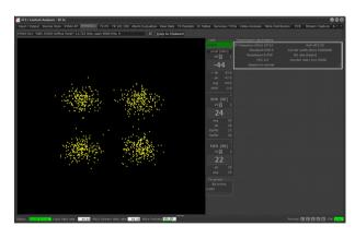
Constellation, Level, MER. SNR and all signalling information can be found here on an easy to read display.
